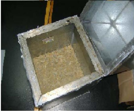
Figura 2: Primary container full of radon source
