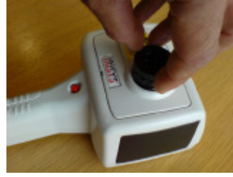
Figure 20 Filter being screwed into place
