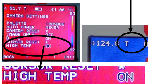
Figure 23 High Temperature on.
