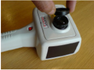
Figure 19 Filter being fitted
